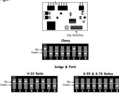
**NOTE:** To ensure proper function of the dip switches, flip each dip switch back and forth once before setting them, even if the dip switches are already set for the application it's being installed on.
